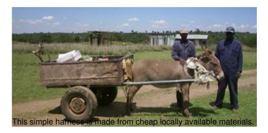
Its main limitation is that the vertical load from the cart is taken on the neck and not the back.
