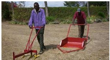
Soil loosener – This tool loosens the hard soil to ease subsequent moving. Several shallow passes are made gradually becoming deeper.
