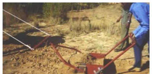
The depth of loading is controlled by the handles. The important features are to maintain a shallow depth so the scoop fills over a distance.
